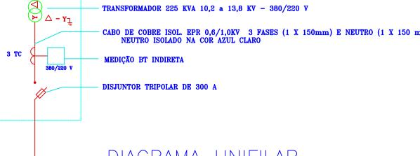
DIAGRAMA UNIFILAR SEM ESCALA
